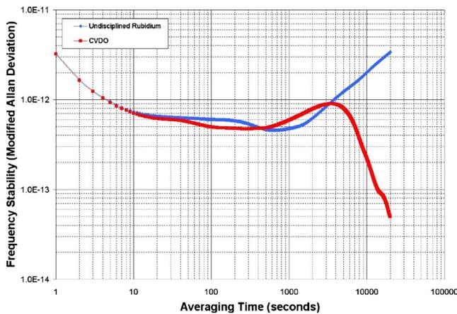
FIG. 5. (Color online) Frequency stability of rubidium CVDO compared to undisciplined rubidium oscillator.
