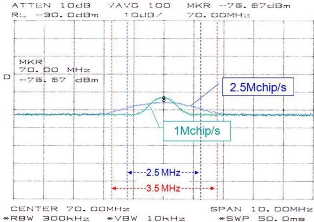
Figure 2. 1 MChip/s and 2.5 MChip/s RX IF spectrum signals.
