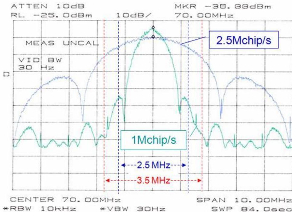
Figure 1. 1 MChip/s and 2.5 MChip/s TX IF spectrum signals.
