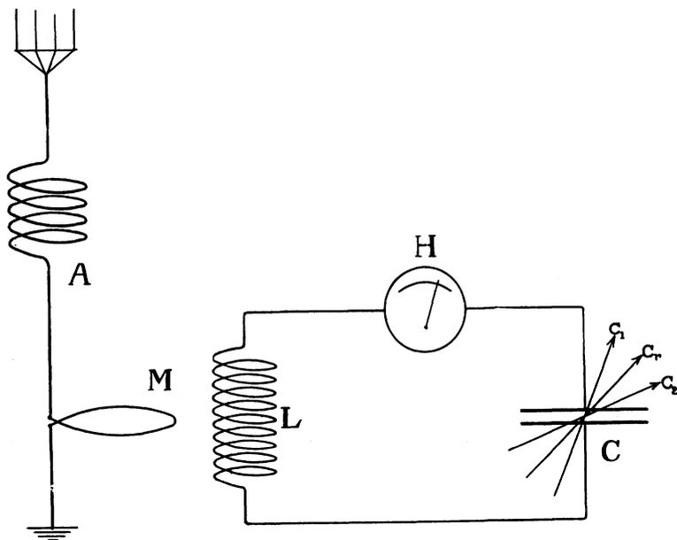
FIGURE 1—Decimeter Circuit Coupled Loosely to the Antenna Circuit of a Transmitter
