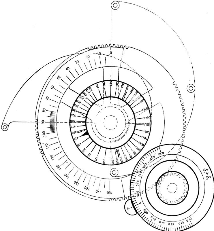
FIGURE 7—Variable Condenser, Showing Gears and Scales Mechanically Attached
