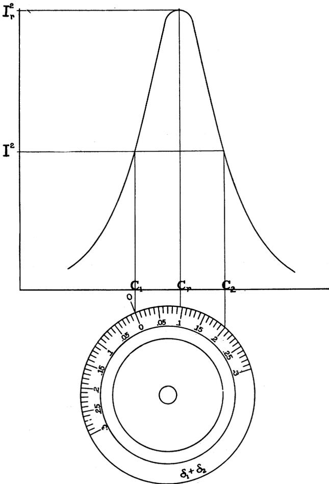
FIGURE 8—Diagram Showing Relation Between Decrement Scale and Resonance Curve
