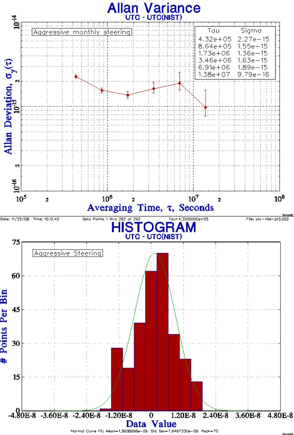
Figure 5. Allan deviation and histogram of time differences with aggressive steering.
