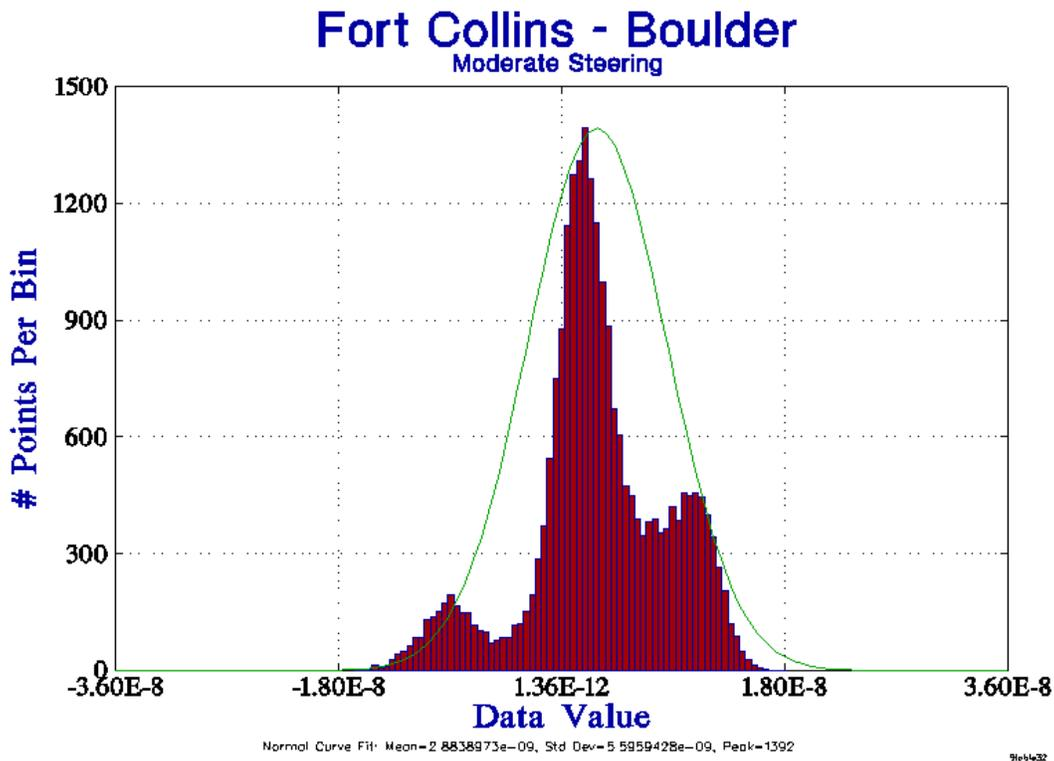
Figure 7. The histogram of the time differences when very slow steering is used.
