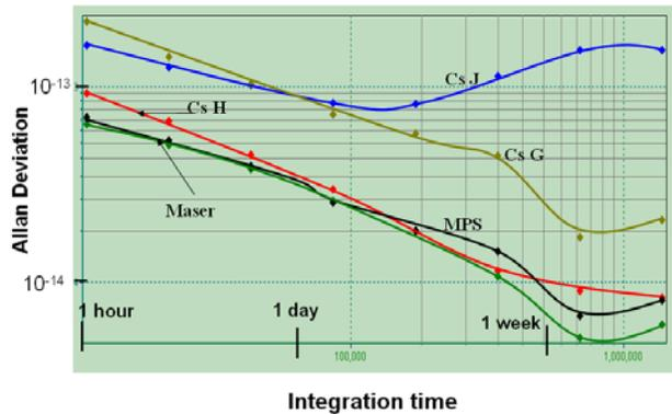
**Figure 5.** Frequency stability of the time difference of participating clocks with respect to the master clock (Cs I). The black line corresponds to the frequency stability of the MPS output.
