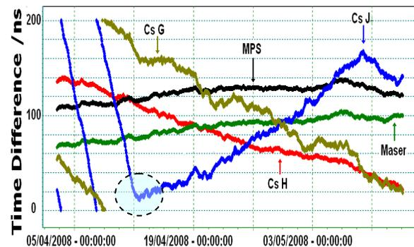
**Figure 3.** Time difference measurement of participating clocks with respect to the master clock (Cs I). The black line corresponds to the MPS output.
