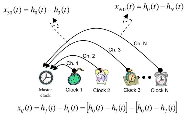
**Figure 1.** Schematic of the time difference measurement system used at CENAM, also referred to as a phase comparator. The system performs one measurement every second.
