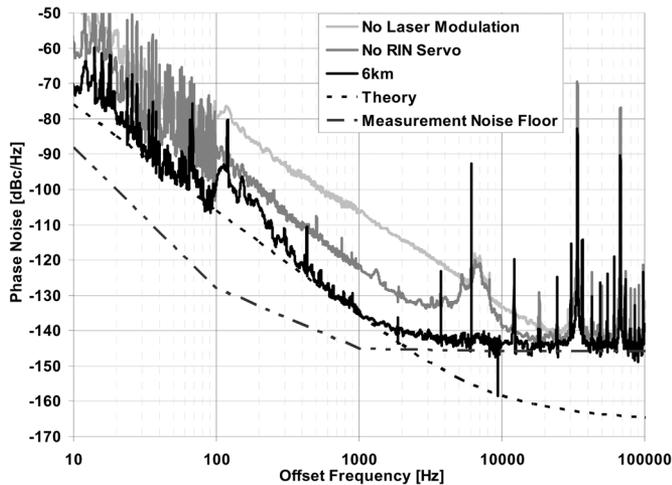
Fig. 8. Phase noise of a 1.25-GHz OEO with 6-km-long fiber. Theory is from Leeson's equation using the photodiode as the dominant flicker source.
