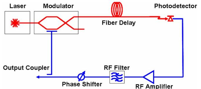
Fig. 1. Basic configuration of an optoelectronic oscillator.
