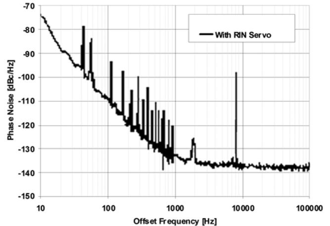
Fig. 6. Improvement in link phase noise after the RIN suppression servo is used.
