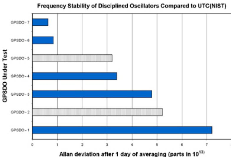
Figure 4. Frequency stability comparison of seven different GPSDOs.
