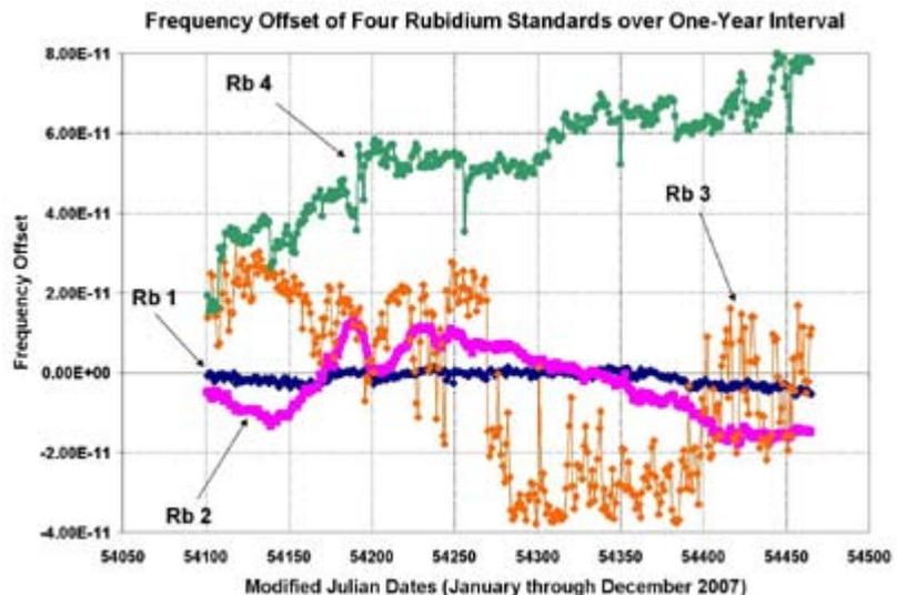
Figure 2. Long-term performance data (one year) from four rubidium frequency standards.
