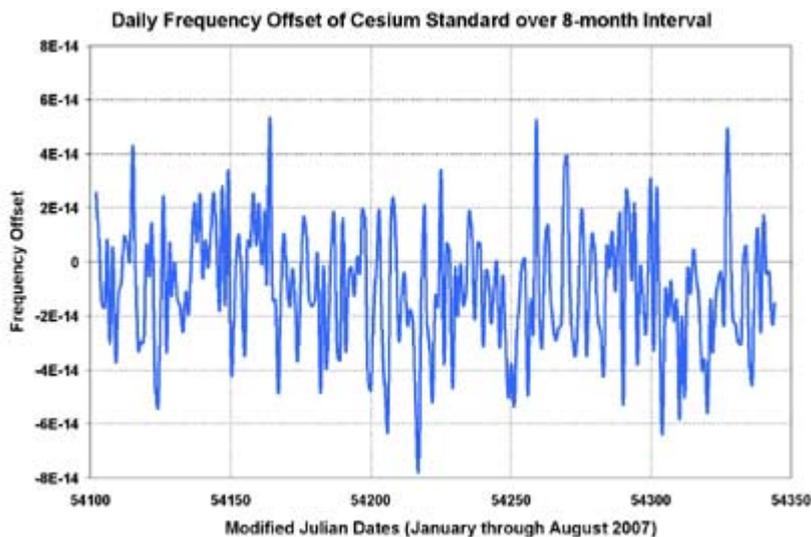
Figure 3. Performance of a cesium frequency standard over an 8-month interval.
