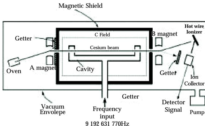
Fig.2. Diagram of a cesium-beam frequency standard using magnetic state-selection and detection. The form of Ramsey interrogation involves a U-shaped microwave cavity (the Ramsey cavity) where the microwave interrogation fields are spatially separated
