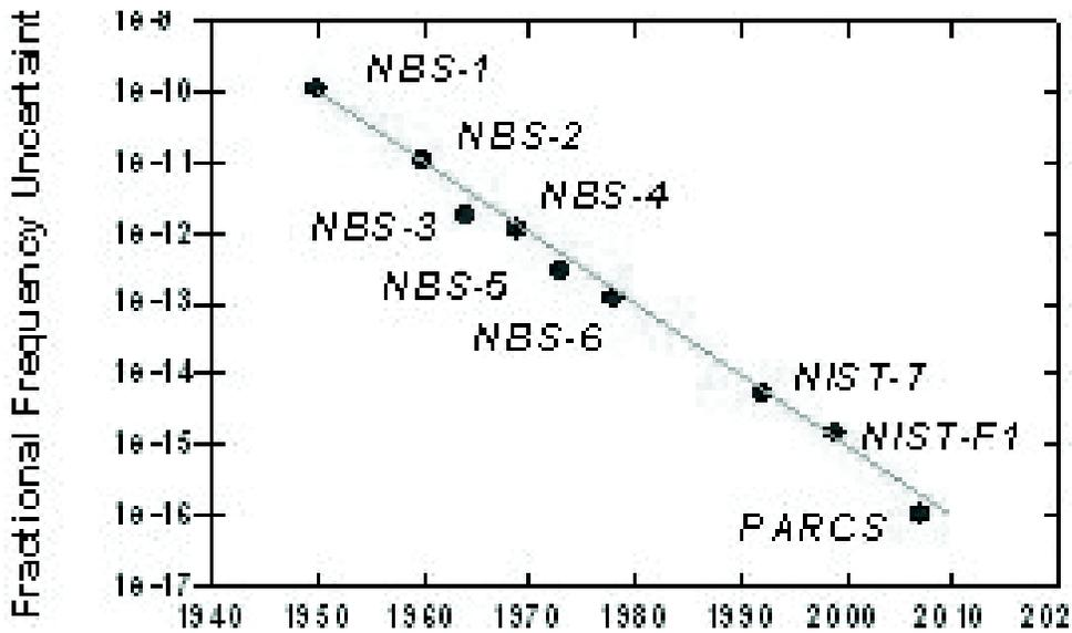
Fig. 1. The inaccuracy of typical primary frequency standards based on the cesium atom hyperfine transition. The slope of the line represents an improvement of about a factor of 10 in accuracy per decade
