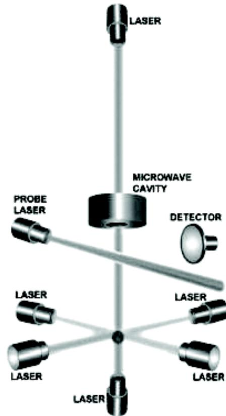
Fig. 3. Schematic diagram of a cesium fountain. Atoms are collected and cooled to  $\approx 1 \mu\text{K}$  at the intersection of six orthogonal laser beams and are tossed vertically with a slight frequency detuning of the vertical lasers. The atoms follow a ballistic trajectory vertically through the microwave cavity (both on the way up and down). The population in each of the two ground-state hyperfine levels is measured by the probe laser after Ramsey interrogation
