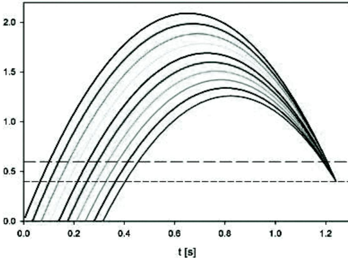
Fig. 4. The multiple ball toss scheme. The horizontal axis in the diagram is the time axis, while the vertical axis is the height above the launch region. As described in the text, the first launched ball goes the highest, while the next ball has an apogee slightly less, and so forth. Finally after a free flight for the first ball of about 1.2 s all of the atoms are in the detection region, where they are detected as a single ball
