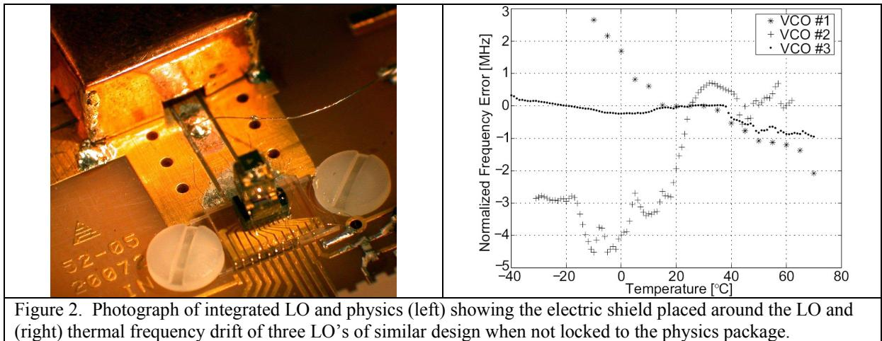
Figure 2. Photograph of integrated LO and physics (left) showing the electric shield placed around the LO and (right) thermal frequency drift of three LO's of similar design when not locked to the physics package.
