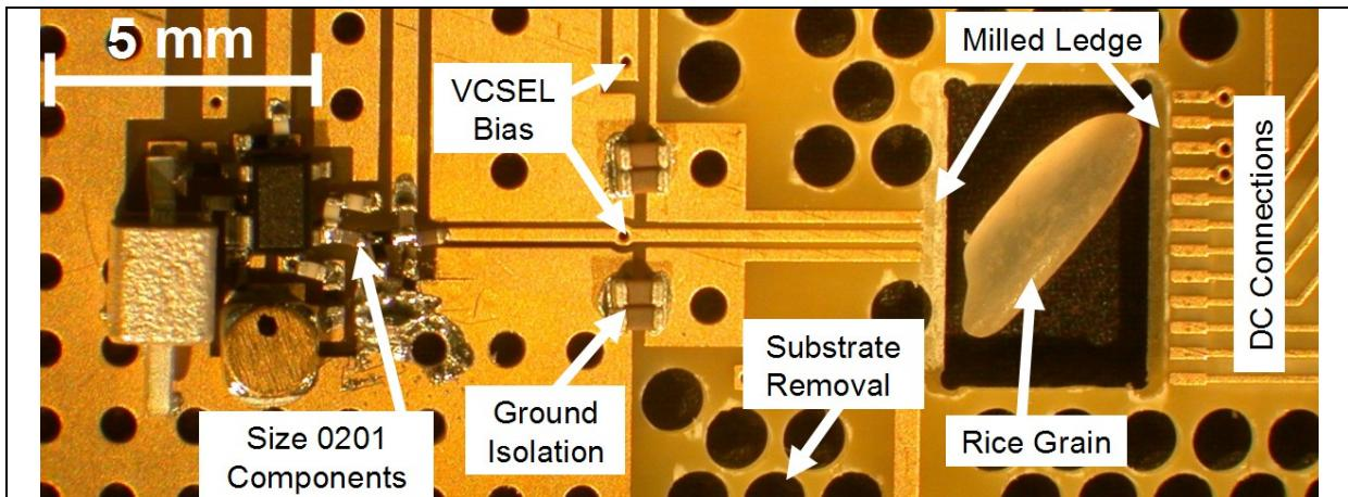
Figure 3. Photograph of an improved integrated system. The physics package is not shown, giving a better view of the board layout. Thermal power losses were reduced by the removal of unnecessary substrate material and by the thinning of circuit traces near the physics package.
