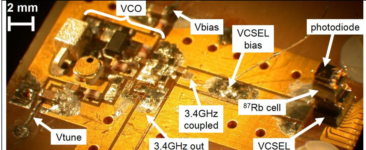
Figure 1. Photograph of the local oscillator (LO) integrated with the physics package. The LO modulates the vertical-cavity surface-emitting laser (VCSEL) at 3.4173 GHz, exciting the coherent-population-trapping (CPT) resonance of gaseous  $^{87}\text{Rb}$  atoms contained in a glass and silicon cell. The photodetector at the top of the physics package receives the laser light and control electronics (not shown) tune the LO to a lock on the CPT resonance.
