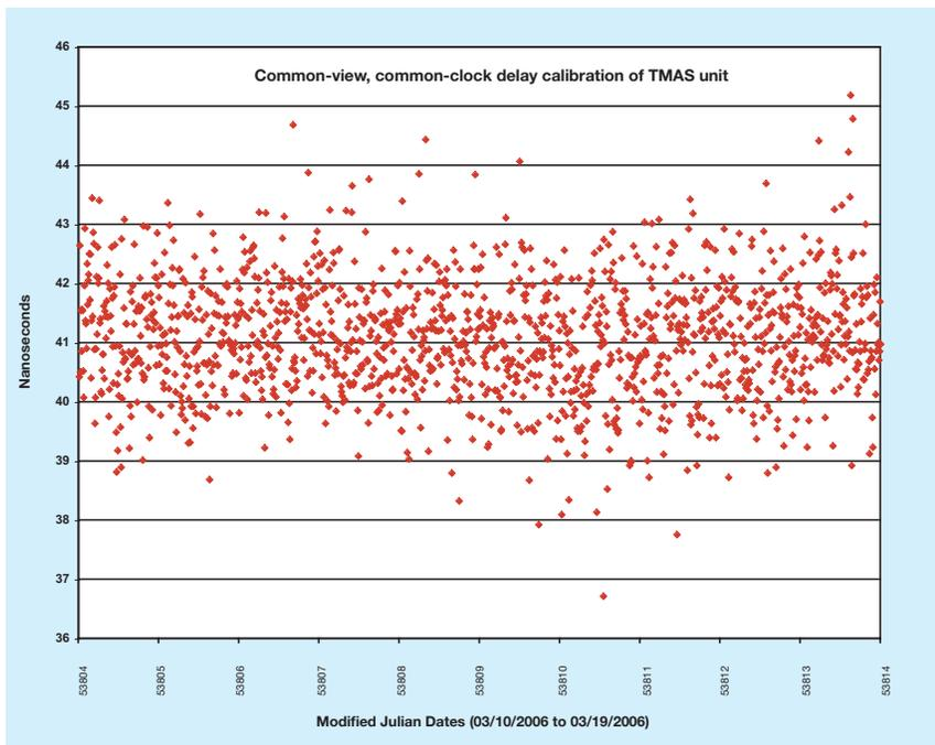
Figure 4. Results of a 10-day TMAS measurement system calibration.
