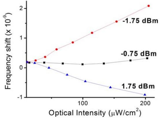
Fig. 3. Frequency shift vs optical intensity for different values of LO-power level
