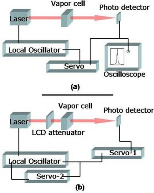
Fig. 1. (a) Schematic of a modulated CPT clock. (b) Schematic of a modulated CPT clock with an additional servo to lock the atomic resonance frequency to the unperturbed atomic resonance frequency.
