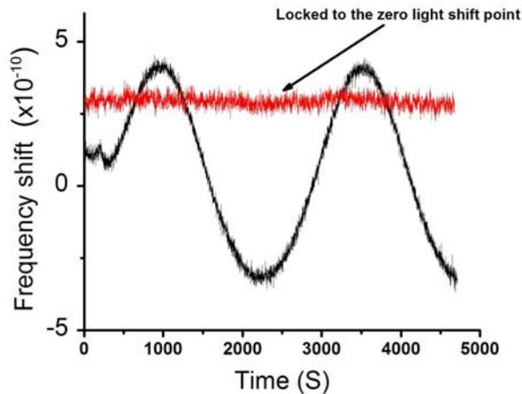
Fig. 4. Clock frequency vs time. The laser temperature was sinusoidally varied with a time period of roughly 2500 s.
