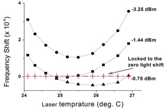
Fig. 2. A plot of clock frequency vs the laser temperature for the conventional case (dots) and when LO-power level is locked to the zero light shifted atomic resonance frequency (+) for different values of LO-power level.
