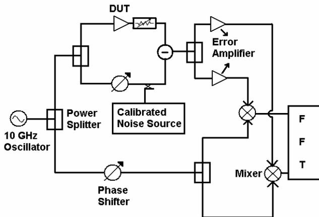
Figure 2. Block diagram of a two-channel carrier-suppressed measurement system.
