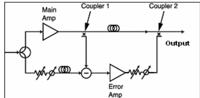
Figure 1. Block diagram of a feed-forward amplifier.
