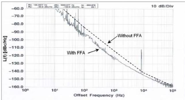
Figure 5. PM noise of NIST air-dielectric cavity oscillator with and without FFA.
