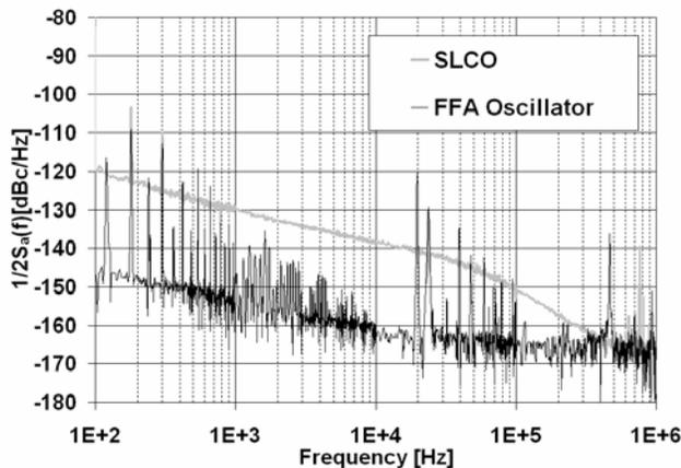
Figure 7. AM noise of FFA oscillator and SLCO.
