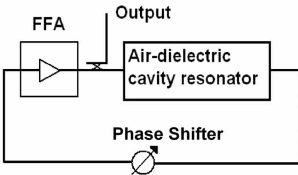
Figure 4. NIST air-dielectric cavity oscillator with FFA.
