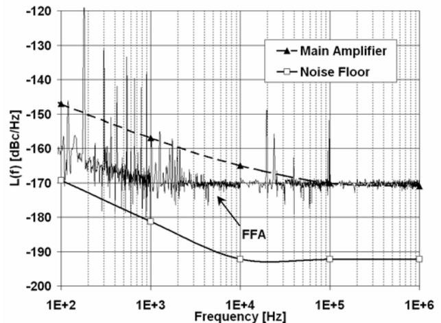
Figure 3. PM noise of main amplifier and FFA.
