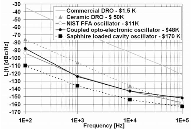
Figure 6. PM noise of different classes of oscillators at 10 GHz.
