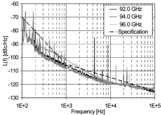
**Figure 5:** PM noise of locked Gunn oscillator at different frequencies. Measured phase noise is combined noise of a pair of similar oscillators. Noise of single oscillator is 0 to 3 dB better than shown.
