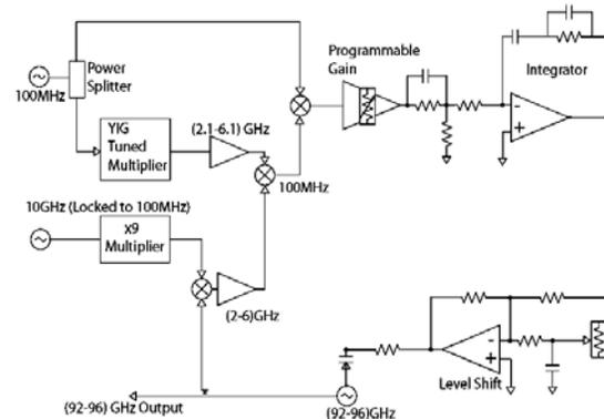
**Figure 3:** Schematic diagram of phase-locked (92-96) GHz Gunn oscillator/synthesizer.
