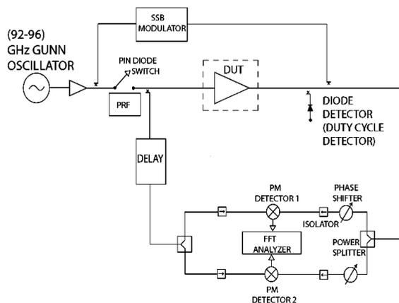
**Figure 1:** The residual PM noise of an amplifier (DUT) is measured with the configuration shown. Mixer and isolator noise in the top PM detectors are uncorrelated with respect to the bottom detectors. The PM noise of the (92-96) GHz oscillator signal is suppressed, since it appears equally at both inputs to the mixers.
