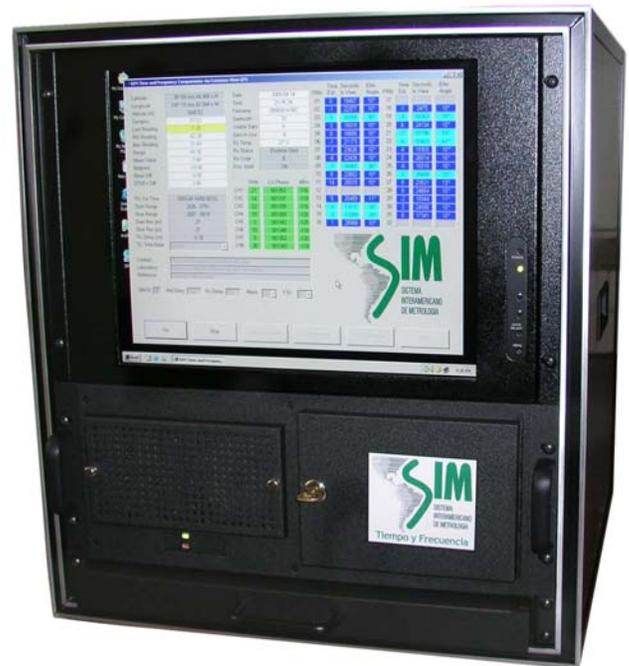
Figure 2. The SIM common-view GPS measurement system.
