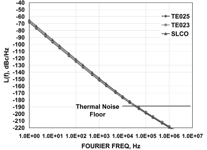
Fig. 2. The computed discriminator noise floors for the CSO using TE023 and TE025 cavities and for the SLCO of Tobar *et al.* [7].
