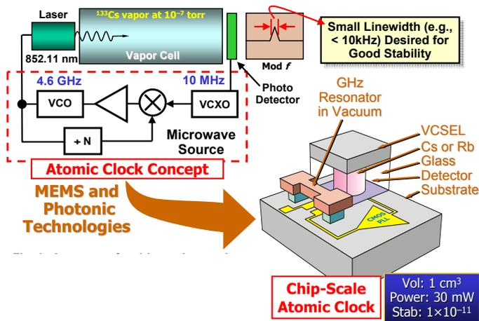
Figure 4.5.3: Anatomy of a chip-scale atomic clock. To date, tiny cells and gigahertz reference resonators have been successfully demonstrated with high Q, and low power oven control has been achieved. Control and oscillator circuit power consumption remain as bottlenecks to the 30mW goal.
