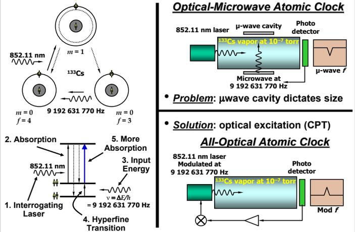
Figure 4.5.2: Physics and implementation strategies for small atomic clocks, where the output frequency is determined by the energy of an atomic transition.
