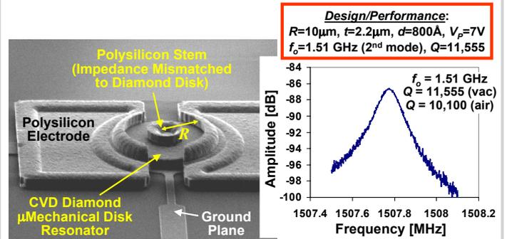
Figure 4.5.4: Scanning electron micrograph (SEM) and measured frequency characteristic for a 1.51-GHz polydiamond micromechanical disk resonator. The measurement was performed without matching to the network analyzer, so the amplitude is not indicative of actual loss.
