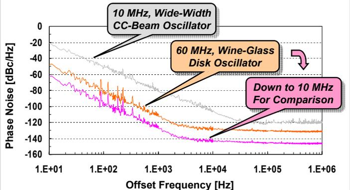
Figure 4.5.6: Measured phase noise density versus carrier offset for the 10MHz CC-beam oscillator of [6] and the 60MHz wine-glass oscillator of Figure 4.5.5, with an extrapolation for the latter down to 10MHz for fair comparison.
