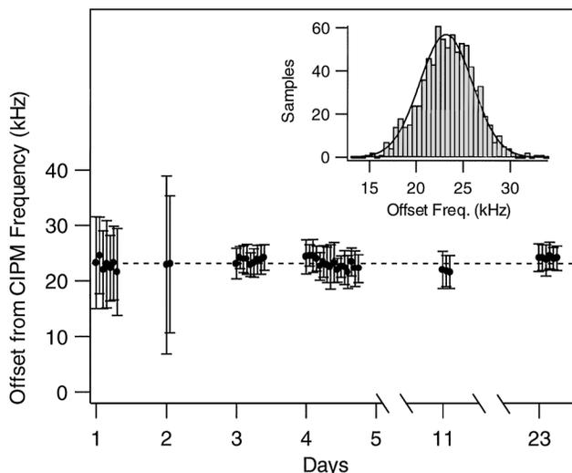
Fig. 3. Summary of measured Nd:YAG frequency  $f_{1064}$  with respect to the CIPM recommendation of 281, 630, 111, 740 kHz. The dashed line is the average of all the plotted points (23.2 kHz). The inset is a histogram of the  $\sim 800$  individual measurements on and after the third day.
