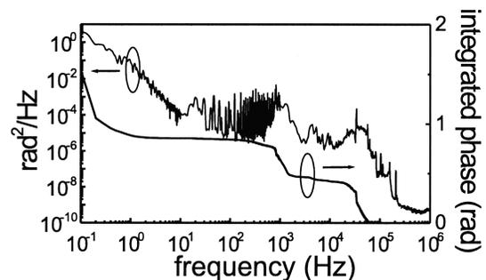
Fig. 2. Left-hand axis, phase-noise power spectral density of the  $\Delta f_0$  beat, equivalent to the phase noise of the optical frequency comb components around 900 nm (333 THz). Right-hand axis, integrated phase noise.
