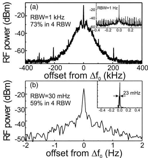
Fig. 1. Heterodyne beat measured around 900 nm between the two FLFCs with  $\Delta f_0 = 101$  MHz. (a) Measurement with a RF spectrum analyzer at 1-kHz RBW. Inset, measurement with 1-Hz RBW. (b) Measurement of the beat mixed to 10 Hz with a fast Fourier transform spectrum analyzer at 30-mHz RBW (inset, with 3-mHz RBW, linear scale). The fraction of overall power contained in the central peaks is indicated.
