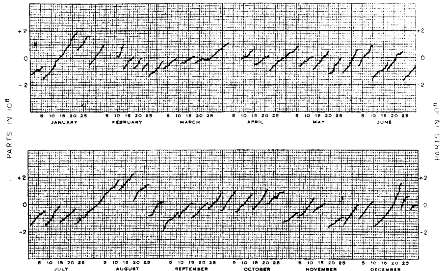
Fig. 3: Graphs of daily frequency errors compared with WWV broadcast by WWVH; discontinuities in trace indicate frequency deviation correction to local generator
