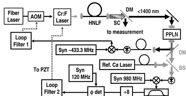
Fig. 1. Schematic of the stabilization scheme for the IR comb: SC, supercontinuum; DMs, dichroic mirrors; Syns, synthesizers; BSs, beam splitters;  $\phi$  det, phase detector; Loop Filters 1, 2, electronic servo filters.
