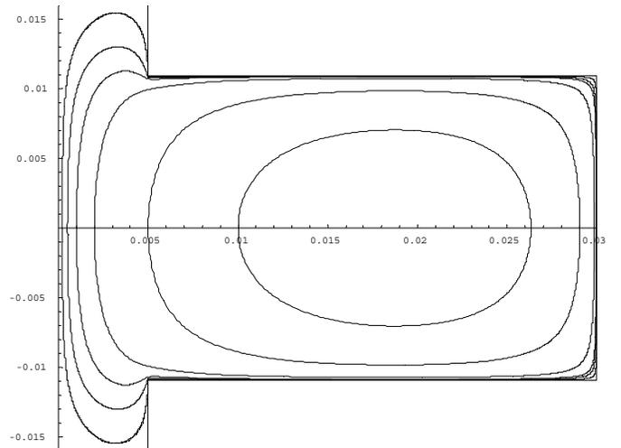
Figure 8. The pattern of the magnetic field within the cavity shown in an  $r$ - $z$  plot. The units on the axis are meters. The density of field lines should not be taken as an indication of the field strength, as the lines plotted were simply chosen for clarity.
