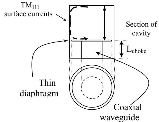
Figure 13. New design of the choke for the cylindrical cavity using a coaxial waveguide with reduced inner conductor radius and a thin diaphragm with a smaller annular gap placed between the cavity and the coaxial waveguide.
