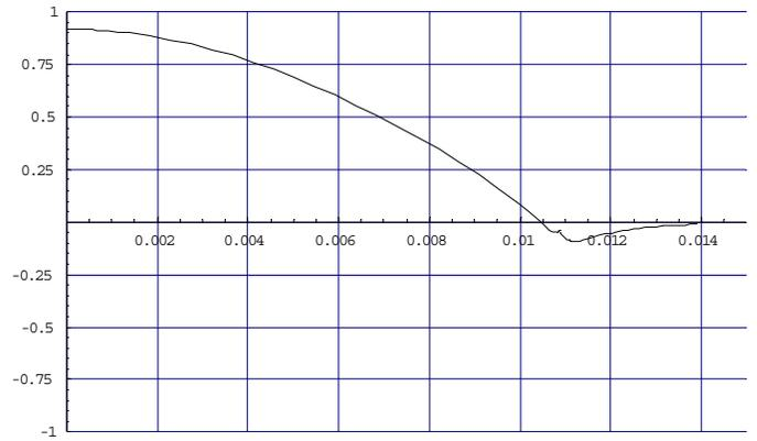
Figure 7. The  $z$  component of the microwave magnetic field plotted as a function of distance from the center of the cavity in the  $z$  direction at  $r = 0.0045$  m (next to the edge of the below-cutoff waveguide). The small discontinuity in the field at  $z \sim 0.011$  m is a result of the previously mentioned Gibbs phenomenon. The field strength is normalized to unity at the center of the cavity,  $r = 0, z = 0$ .
