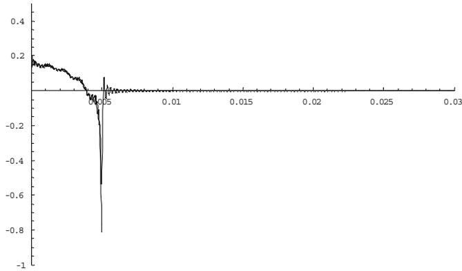
Figure 5. The field solutions just inside the below-cutoff waveguide and just inside the cavity ( $z = L/2 \pm \epsilon$ ) are overlaid. The large overshoot of the solutions at the edge of the below-cutoff waveguide is a Gibbs phenomenon. The “diffraction” pattern caused by the below-cutoff waveguide edge can be seen in the four or five wiggles between  $r = 0$  and  $r = 0.005$  m.
