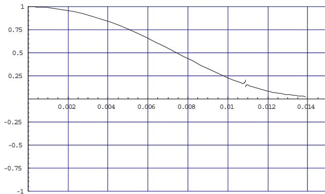
Figure 6. The on-axis ( $r = 0$ )  $z$  component of the microwave magnetic field plotted as a function of distance from the center of the cavity in the  $z$  direction. The small discontinuity in the field at  $z \sim 0.011$  m is a result of the previously mentioned Gibbs phenomenon. The field strength is normalized to unity at the center of the cavity,  $r = 0, z = 0$ .
