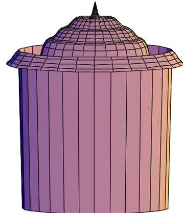
Figure 4. The field at the endcap of the microwave cavity plotted only over the below-cutoff waveguide ( $0 < r < 0.005\text{m}$ ,  $z = L/2$ ). The effect of the below-cutoff waveguide can be clearly seen as a large field reversal at this point. The diffraction rings can also be seen in the "staircase-like" behavior of the field strength.
