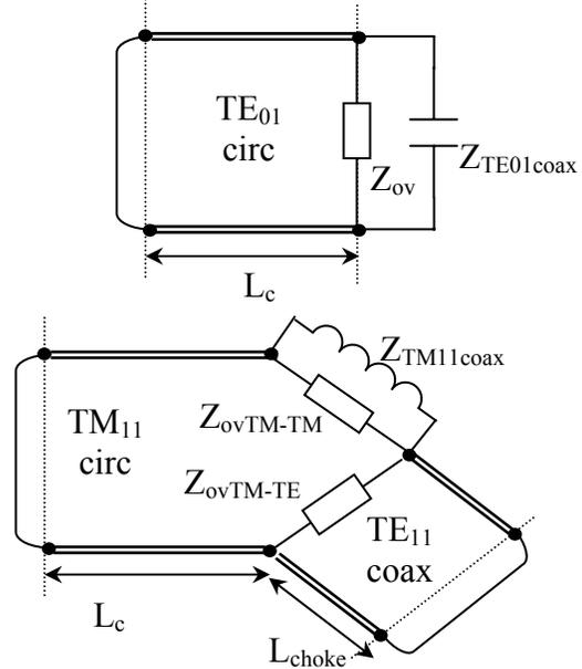
Figure 12. Transmission-line equivalent circuits for TE<sub>01</sub> (top) and TM<sub>11</sub> (bottom) modes inside the cavity, when loaded with a simple choke with a 1mm-annular gap.
