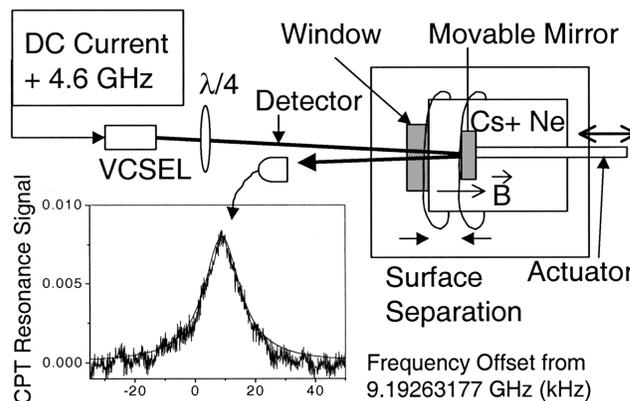
Fig. 1. Experimental setup. The resonance signal is normalized to the Doppler background absorption, measured at  $1.1\ \text{mW}/\text{cm}^2$  and a gap size of  $580\ \mu\text{m}$ .
