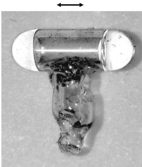
FIG. 3. A cell fabricated from a hollow-core Pyrex fiber using CO 2 laser fusion. The arrow indicates a distance of 1 mm.
