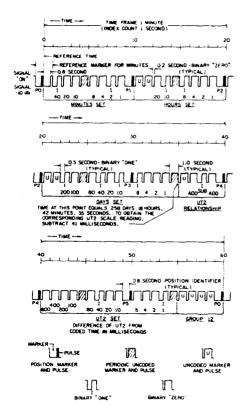
Time-scale representation of carrier level-shift modulation. BCD code gives time, day, and difference between WWVB and UT2 time scales.
