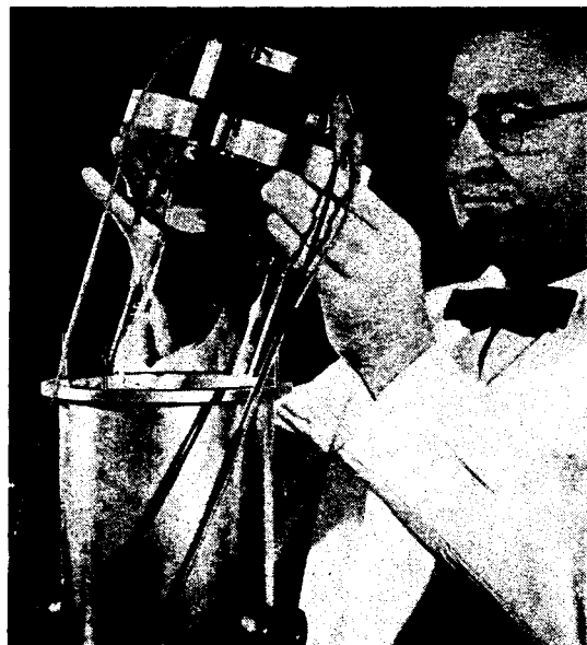
1,650,763.73 wavelengths in vacuo of a specified transition in the isotope krypton-86 now define the meter. The lamp used to produce these wavelengths is shown being placed in a dewar flask. U-shaped tube contains krypton gas in which continuous electric discharge is maintained.
