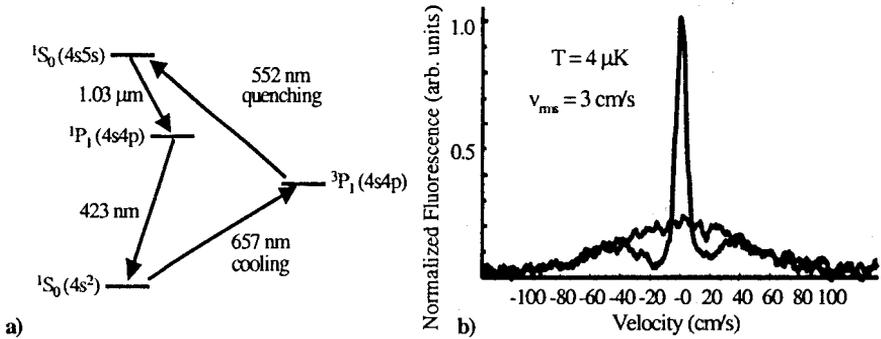
Figure 5. (a) Relevant energy levels for cooling. (b) Velocity distribution of atoms before and after 15 chirped and 10 stationary second-stage cooling cycles. Each cycle consisted of two counter-propagating, temporally separated,  $5 \mu\text{s}$  red pulses followed by  $20 \mu\text{s}$  of 552 nm light. A  $40 \mu\text{s}$  post cooling pulse of 552 nm light was used to pump the remaining atoms back to the ground state. See Ref. [16].
