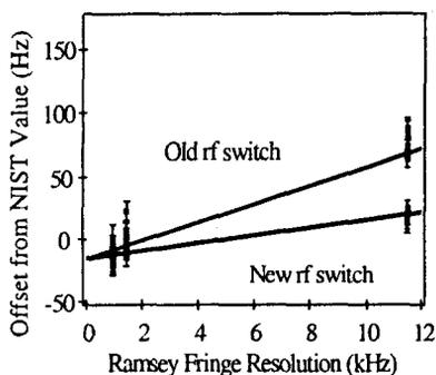
Figure 4. Resolution-dependent shift of the Ca standard frequency. This shift is reduced with improved switching electronics.
