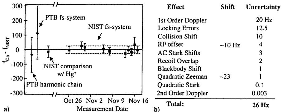
Figure 3. (a) Comparison of Ca absolute frequency measurements. (b) List of systematic uncertainties.
