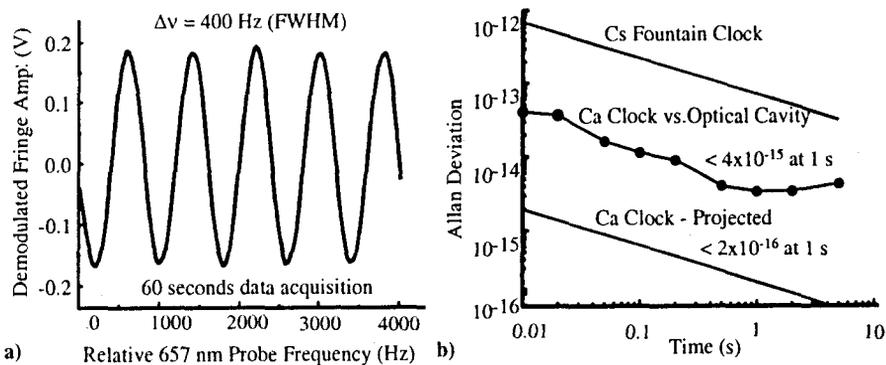
Figure 2. (a) Bordé-Ramsey fringes at the natural linewidth of the “clock” transition. (b) Ca short-term instability measured against an optical cavity.
