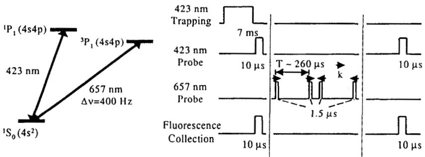
Figure 1. (a) Relevant Ca energy levels. (b) Timing diagram for spectroscopy on the "clock" transition.
