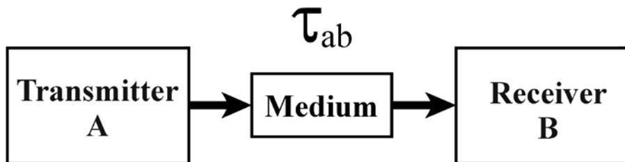
The delay,  $\tau_{ab}$ , over a transmission path is at least 3.3 microseconds per kilometer. If high accuracy time transfer is desired in a one-way system the physical locations (coordinates) of the two clocks must be known so that the path delay can be calculated. For frequency transfer, only the variability of the delay (the path stability) is important.
