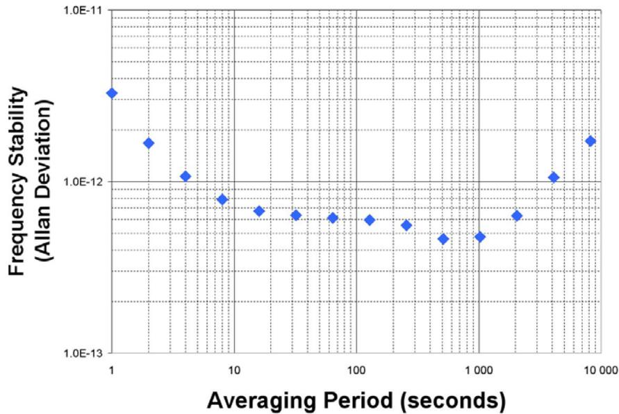
The Allan deviation is also used to identify types of oscillator and measurement system noise. The slope of the Allan deviation line can identify the amount of averaging needed to remove these noise types, as shown in the graph below. Note that the Allan deviation does not distinguish between white phase noise and flicker phase noise.
