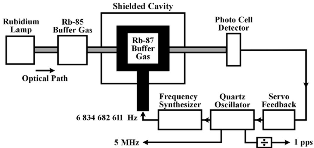
Rubidium oscillators continue to become smaller and less expensive, and offer perhaps the best price to performance ratio of any oscillator. Their long-term stability is much better than that of a quartz oscillator and they are also smaller, more reliable, and less expensive than cesium oscillators.
