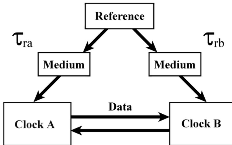
Common-view directly compares two clocks or oscillators to each other. Errors from the two paths ( $\tau_{ra}$  and  $\tau_{rb}$ ) that are common to the reference cancel out, and the uncertainty caused by path delay is nearly eliminated. The result of the measurement is (Clock A - Clock B) - ( $\tau_{ra}$  -  $\tau_{rb}$ ).
