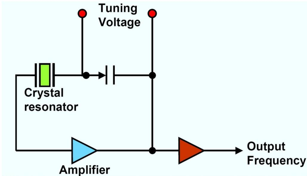
The rate of expansion and contraction is the resonance frequency, and is determined by the cut and size of the crystal. The output frequency of a quartz oscillator is either the fundamental resonance or a multiple of the resonance, called an overtone frequency. A typical  $Q$  for a quartz oscillator ranges from  $10^4$  to  $10^6$ . The maximum  $Q$  for a high stability quartz oscillator can be estimated as  $Q = 1.6 \times 10^7 / f$ , where  $f$  is the resonance frequency in megahertz.
