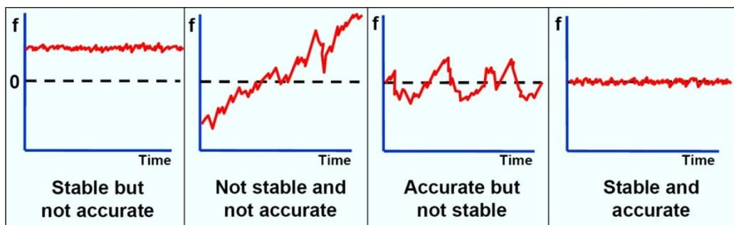
The term uncertainty is usually preferred to accuracy when a quantitative measurement result is reported. Accuracy is often used in a qualitative sense. For example, we might say that an accurate time measurement was made with an uncertainty of 1 microsecond.
