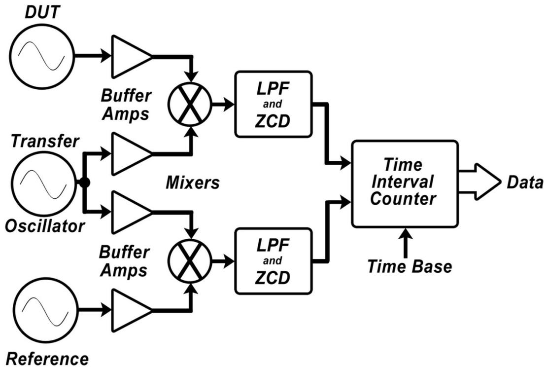
The resolution of a DMTD system is determined by the resolution of the TIC or the time-tagging hardware, divided by the heterodyne factor. For example, if the TIC resolution is 100 ns and the heterodyne factor is  $10^6$  (based on a 10 MHz nominal frequency and a 10
