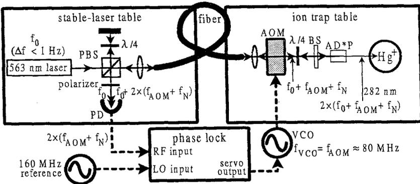
Figure 4. Fiber-noise cancellation scheme. A phase-locked loop controls the deflection frequency  $f_{\text{AOM}}$  of an AOM to suppress the frequency noise  $f_N$  on the light caused by the optical fiber. BS, beam splitter; PBS, polarizing beam splitter.
