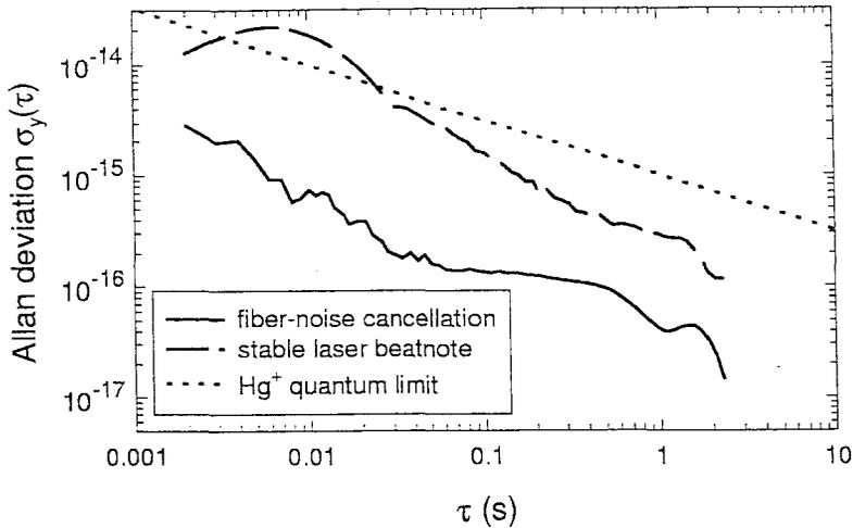
Figure 5. Fractional frequency instability introduced by our fiber link with fiber-noise cancellation. The Allan deviation measured for the incident laser light is  $\approx 10$  times larger than the instability introduced by the actively corrected fiber link.
