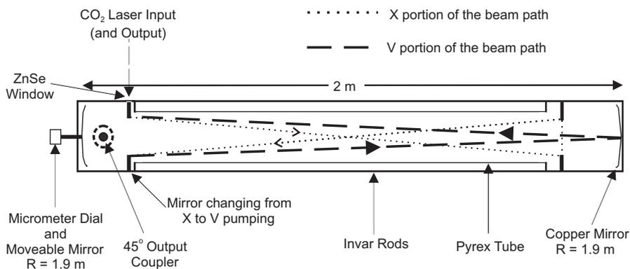
**FIGURE 1** Side view of the X–V mirror geometry used in the optically pumped molecular laser system
