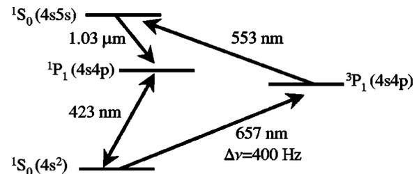
FIG. 1. Relevant energy level diagram for QNLC in  $^{40}\text{Ca}$ . The 553-nm quenching beam transfers population from the long-lived ( $400 \mu\text{s}$ )  $^3P_1(4s4p)$  state to the ground state via the short-lived (30 ns)  $^1S_0(4s5s)$  state.
