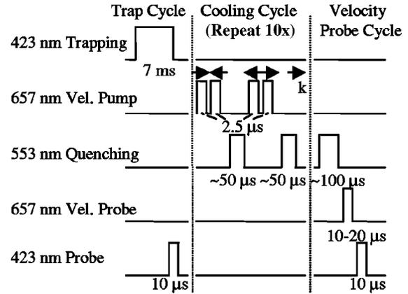
FIG. 2. Timing diagram for our experimental realization of QNLC. Arrows represent the relative direction of the  $k$  vector for each pulse. For short quenching times it would be more efficient to use a copropagating 553-nm pulse after each 657-nm pulse.
