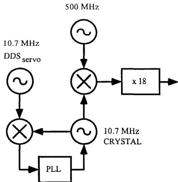
Figure 3: Details of Microwave Synthesis Chain. A 10.7 MHz “clean-up” oscillator is phase locked to the DDS unit in order to reduce the levels of spurious sidebands.
