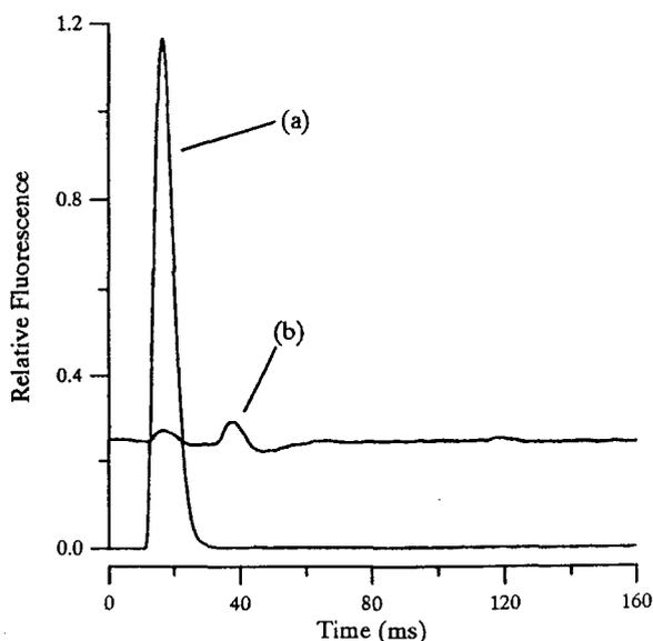
Figure 5: Effect of Synthesizer Phase Transients. Trace (a): Normal slow square wave FM transient due to the atomic transit time distribution. This trace was taken with the frequency servo enabled, thus the steady state fluorescence levels before and after the transient are equal. Trace (b): Effect of DDS phase transients (figure 4(a)) on atomic beam fluorescence. Trace (b) has been offset for clarity.
