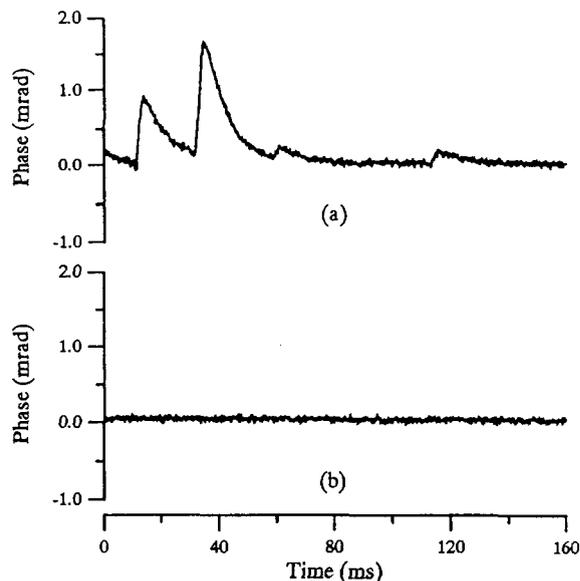
Figure 4: Phase Transients Due to Computer Control. Trace (a): phase transients occurring after frequency control command is sent to synthesizer at  $t = 0$  ms. Trace (b): suppression of phase transients when phase locked loop is disabled.
