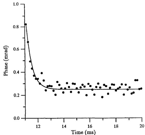
Figure 6: PLL Error Signal During Frequency Step. Dots: Measured phase error after the DDS was instructed to perform a 54 Hz step (the peak to peak modulation amplitude). Solid Line: Exponential fit to the data.
