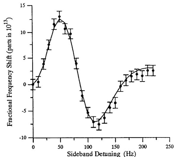
Figure 2: Frequency Shift Due to Sideband Pulling. Solid line is the theoretical calculation. Dots are the experimental measurements. Carrier power: -2.5 dB relative to optimum power; lower sideband: -29 dBc; upper sideband: -66 dBc. Experiment duration: 300 seconds per point.
