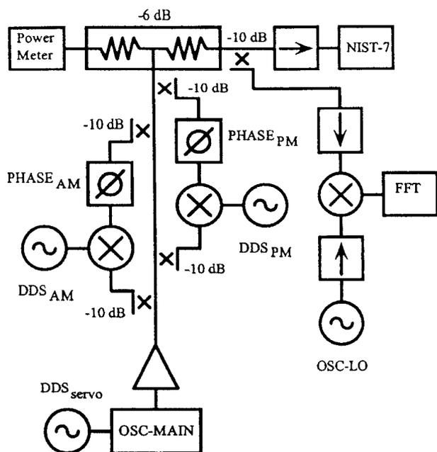
Figure 1: Single Sideband Modulator.
