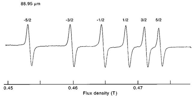
FIG. 1. Part of the far-infrared LMR spectrum of the Al atom recorded with the 88.95- $\mu\text{m}$  laser line of  $^{13}\text{CH}_3\text{OH}$  in perpendicular polarization. The output time constant of the lock-in amplifier was 0.1 s. The six-line pattern arises from the nuclear hyperfine structure for the  $^{27}\text{Al}$  nucleus ( $I = \frac{5}{2}$ ). The transitions obey the selection rule  $\Delta M_J = 0$ ; each line is labeled by the value of  $M_J$  involved.
