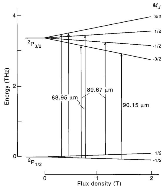
FIG. 2. Energy-level diagram for the Al atom in its ground  $^2P$  state, at zero field and in the presence of an applied magnetic field. The Zeeman splittings are exaggerated for the sake of clarity. The detected transitions are indicated at the observed magnetic fields.
