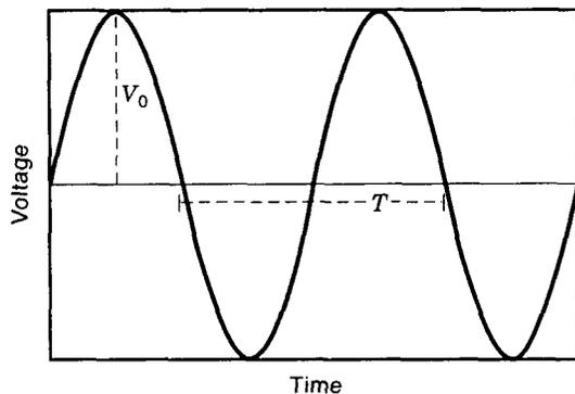
Figure 1. Ideal output voltage of a frequency standard.
