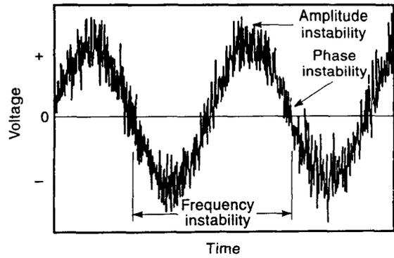
Figure 2. Output voltage of a noisy signal.
