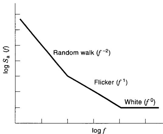
Figure 5. AM noise characteristics of a source.
