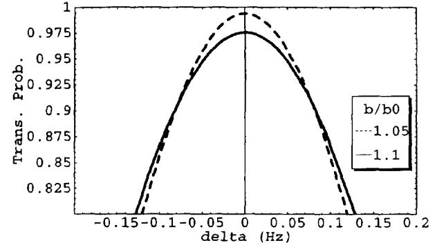
Figure 3. Fringe crossing at two microwave field values illustrating the approximate location of power insensitive detuning point of frequency for a  $\text{TE}_{01,13}$  cavity.
