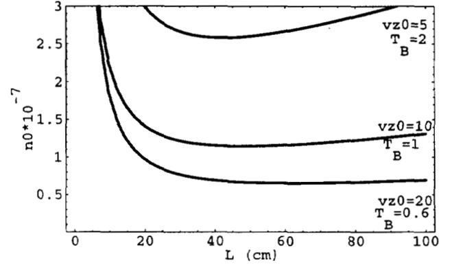
Figure 4. Required number of atoms at launch in  $m_F = 0$  state for  $10^{-14}$  stability in 1 s for a Ramsey cavity.  $L$  is the end-to-end cavity length. Three launch velocities are shown with corresponding times between ball launches  $T_B$ .
