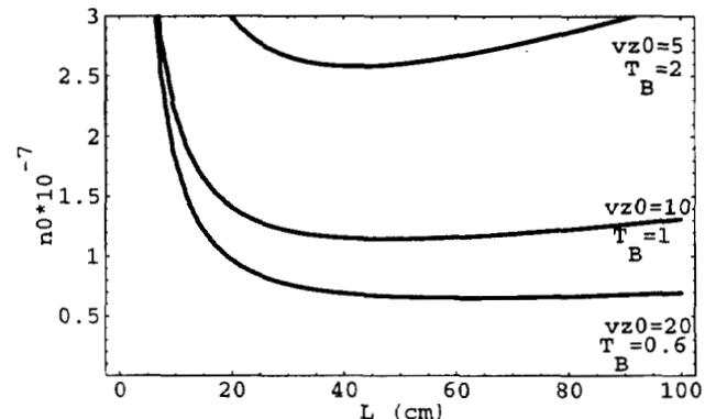
Figure 4. Required number of atoms at launch in  $m_F = 0$  state for  $10^{-14}$  stability in 1 s for a Ramsey cavity. L is the end-to-end cavity length. Three launch velocities are shown with corresponding times between ball launches  $T_B$ .
