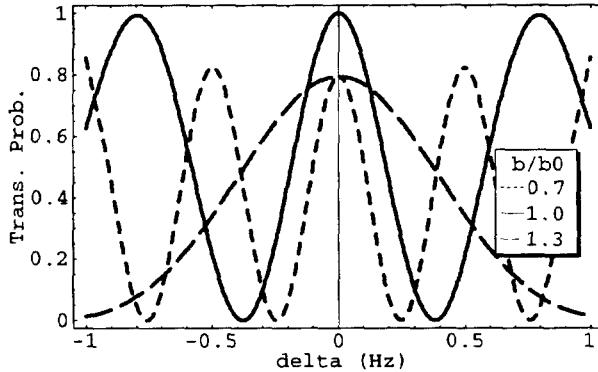
Figure 2. Fringes for a  $\text{TE}_{01,13}$  cavity at three microwave field strengths vs. detuning,  $\delta$ . The field for unit transition probability is  $b_0$  for velocity  $v_{z0}$ . Parameters are given in the text.
