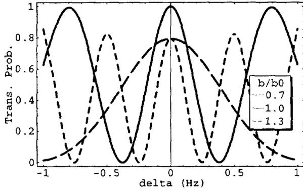
Figure 2. Fringes for a  $TE_{01,13}$  cavity at three microwave field strengths vs. detuning,  $\delta$ . The field for unit transition probability is  $b_0$  for velocity  $v_{z0}$ . Parameters are given in the text.
