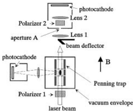
FIG. 1. Schematic diagram (not to scale) for detection of Bragg scattering from an ion cloud, shown as a small prolate spheroid, inside a Penning trap. An  $f/5$  imaging system (left) monitors the shape of the cloud, thereby giving the ion density. The diffraction pattern is relayed to the upper photocathode, filtered by a small aperture (A) and crossed polarizers, as described in the text.
