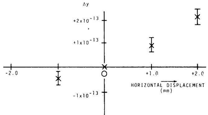
Fig. 2. Plot of relative output frequency versus detector position. On the vertical scale is plotted  $\Delta y \equiv$  fractional frequency offset relative to the geometrically aligned position. On the horizontal scale is plotted relative distance that the detector is moved from the geometrically aligned position.
