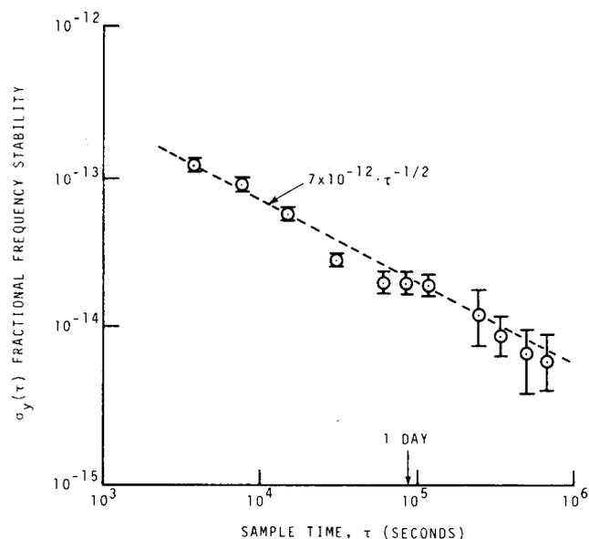
Fig. 1. Measured stability of NBS-4 from December 1975 to January 1976. (bandwidth = 10 Hz).
