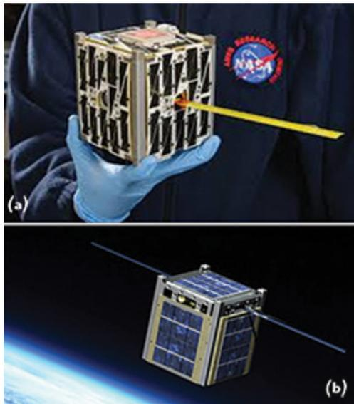
Figure 8 CubeSat hardware (a) and CubeSat in low-Earth orbit (b) (courtesy NASA).<sup>20</sup>
